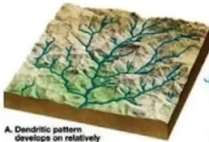
A. Dendritic pattern develops on relatively uniform bedrock
